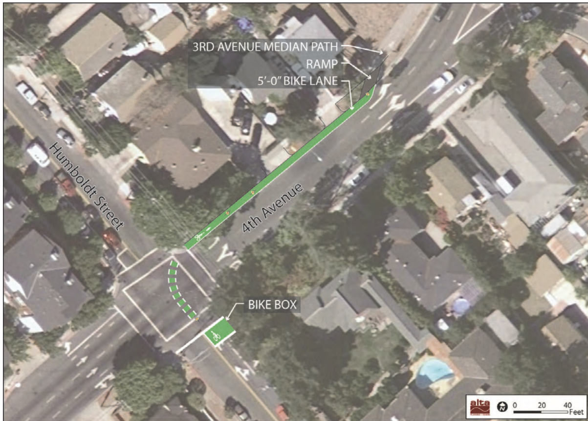
Figure G-8: Proposed Humboldt Street and 4th Avenue Bike Box and Green Bike Lane
