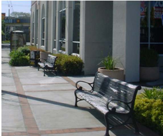
Figure 3.74 Street benches should be made from steel or heavy wood slats for strength and durability.
