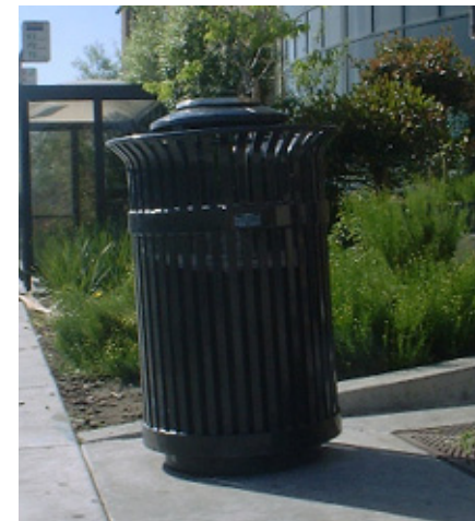
Figure 3.77 Trash receptacles should have steel slats for durability as well as side access for ease of emptying.
