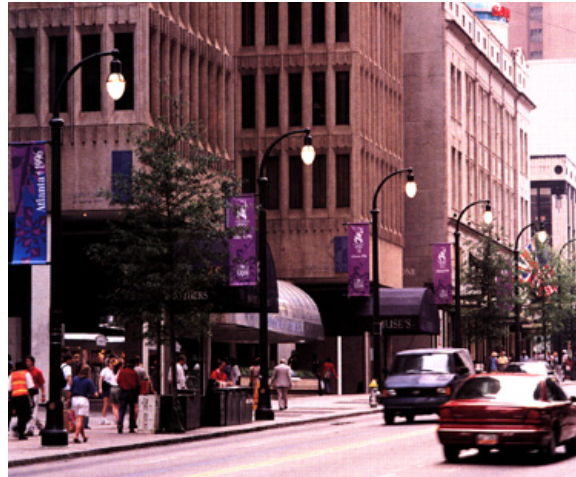
Figure 3.44 Holophane Atlanta Series pole and bracket with a Memphis Series Teardrop luminaire and banner attachment.
