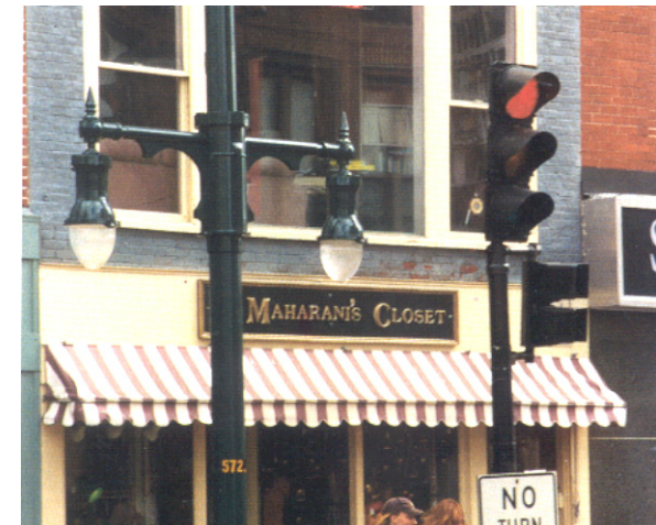
Figure 3.47 Close up of the Holophane Pedestrian Series luminaires showing custom arm brackets and the West Liberty Style decorative arm fitter above the luminaires.
