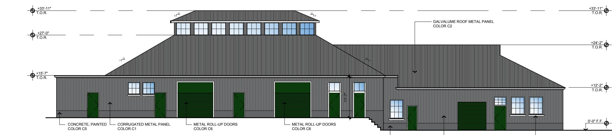
**BUILDING A PROPOSED EAST ELEVATION** 4
