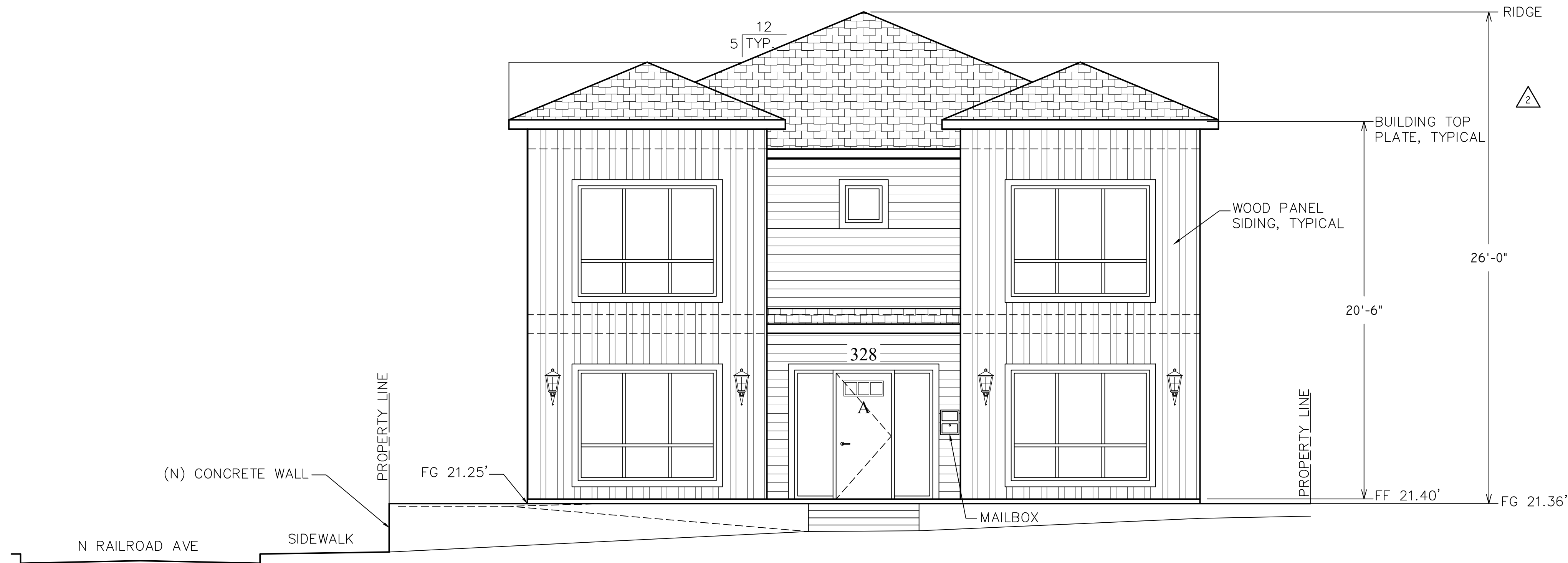
PROPOSED NORTH/ TILTON AVE ELEVATION SCALE: 1/4" = 1'-0"
