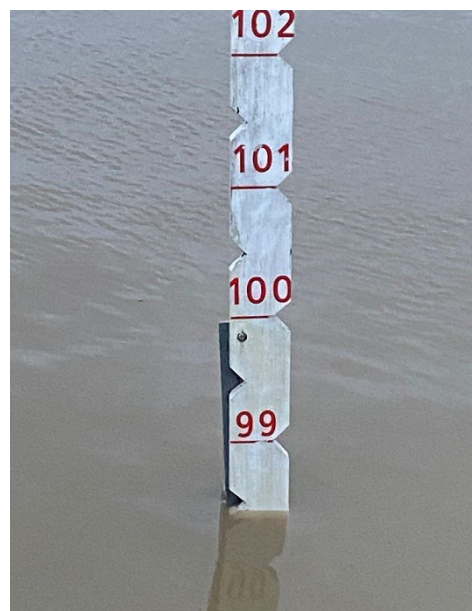
Figure 10: Staff Gage During the Storm, Reading Approximately 98.4 feet CSM
