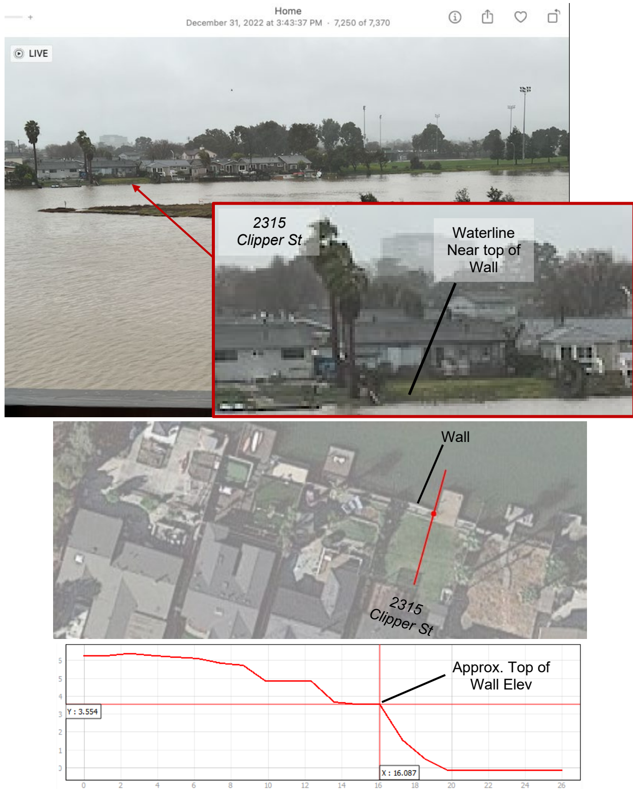
Figure 22: Photo of Lagoon Island and South Bank from a Residence on the Northern Shore of the Lagoon (Top) Over Satellite Image and 2017 LiDAR Profile (Bottom)
