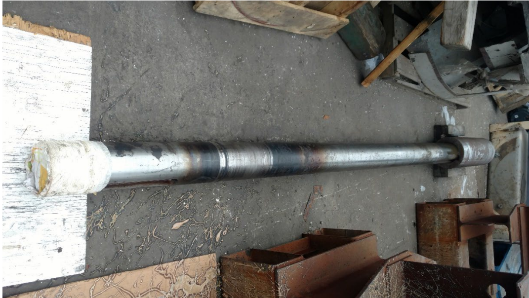
Pump shaft with heat discoloration
