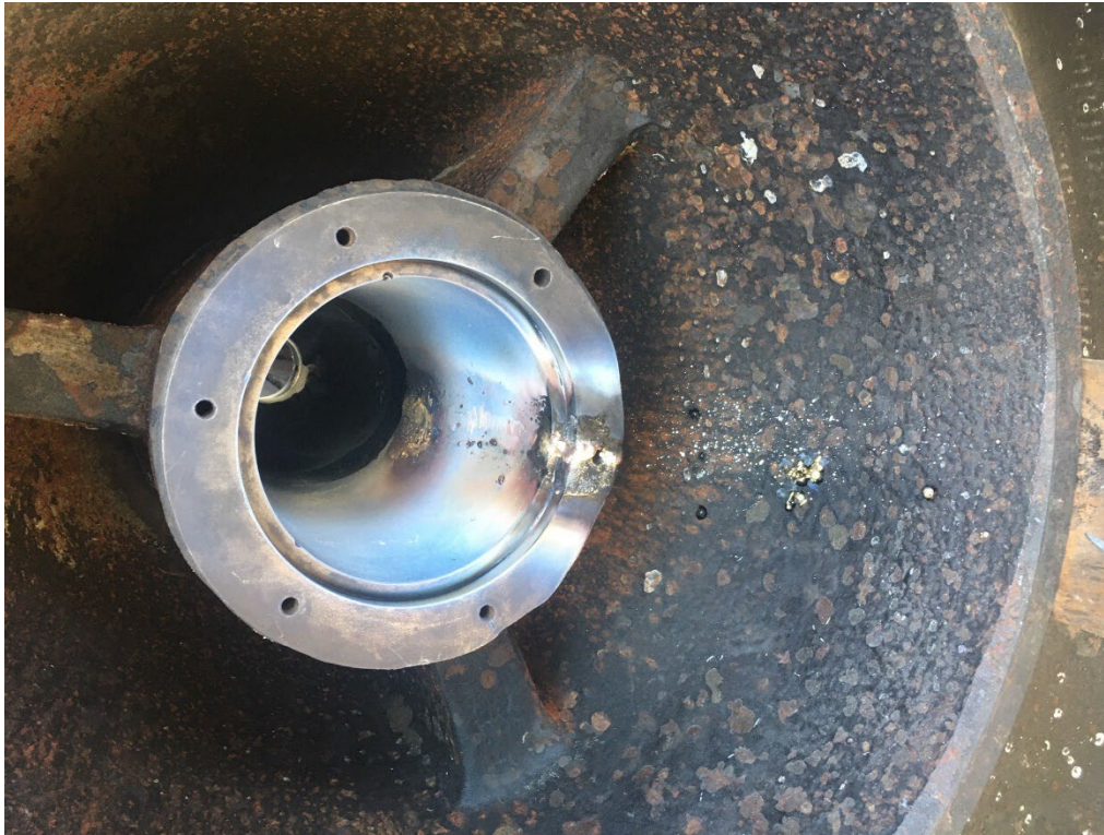
Pump suction bell bearing housing crack repair
