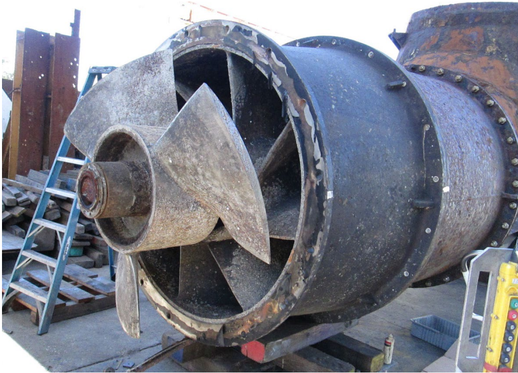
Pump propeller w/ broken pump shaft visible
