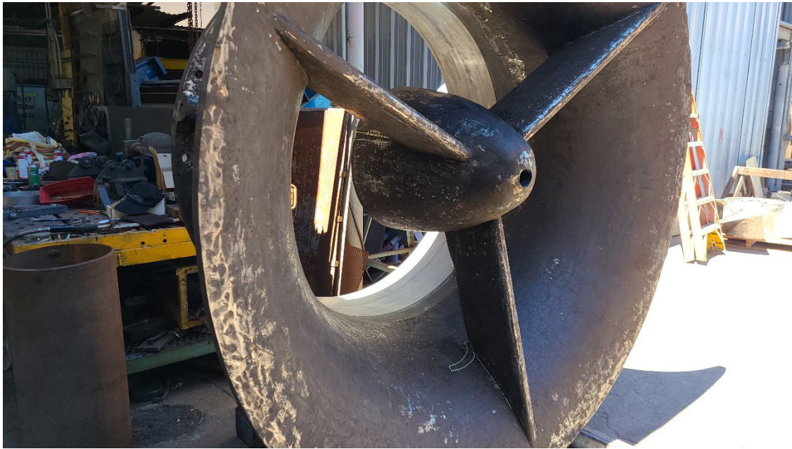
Pump suction bell and bearing housing w/ cracks highlighted for repair
