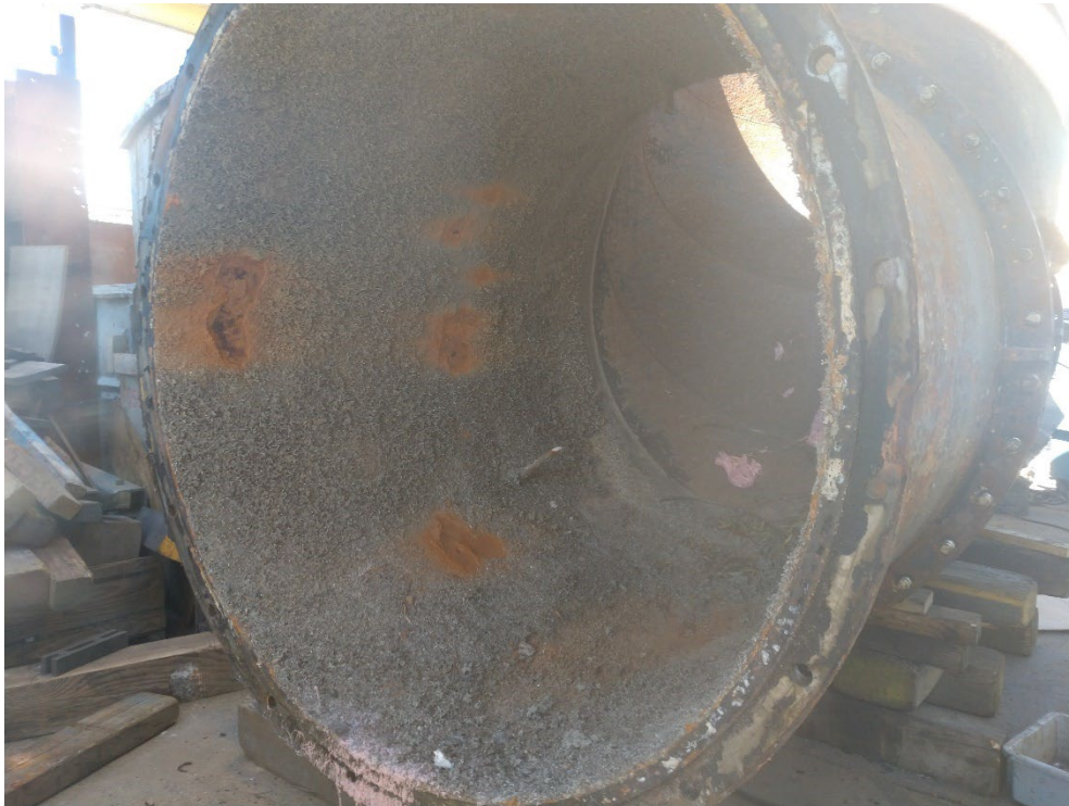
Pump discharge elbow w/ visible corrosion (full penetration)
