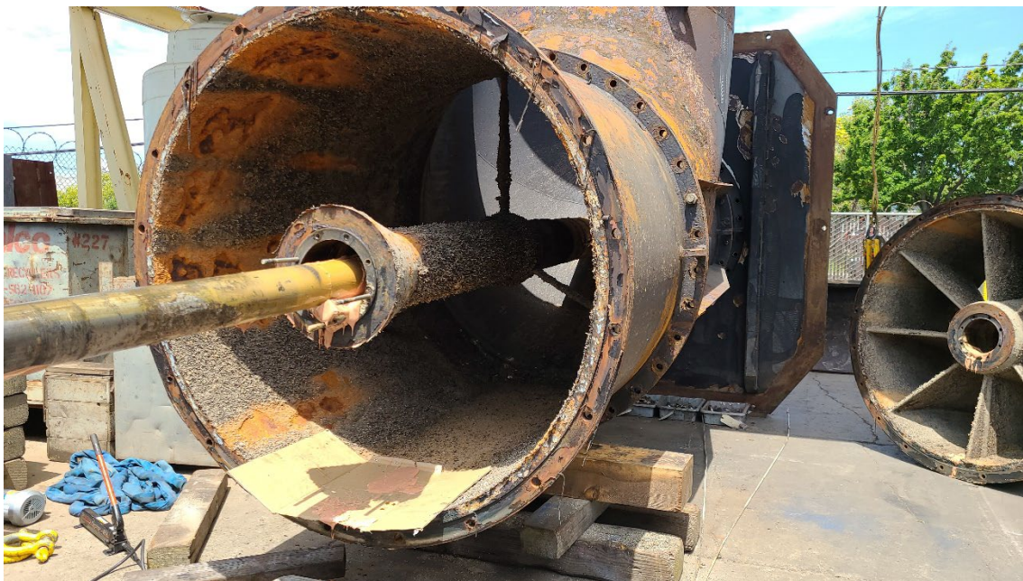
Pump column and shaft enclosure tube w/ visible corrosion
