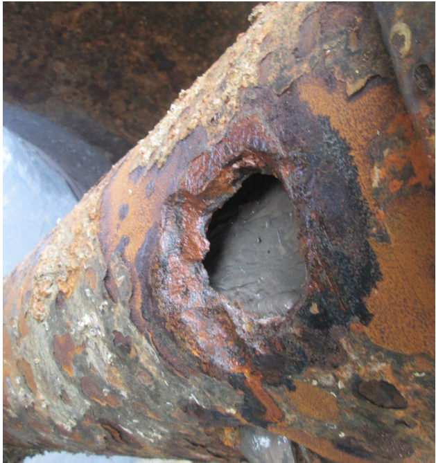
Pump shaft enclosure tube corrosion (full penetration)
