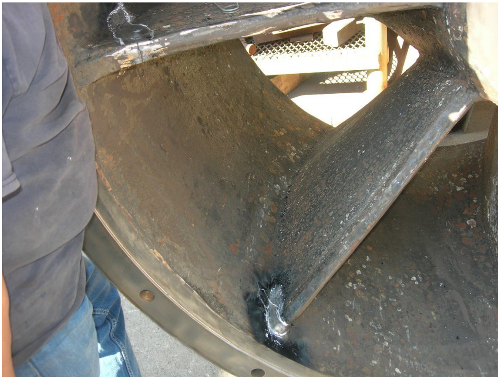
Pump diffuser section vane cracks (preparation for welding)
