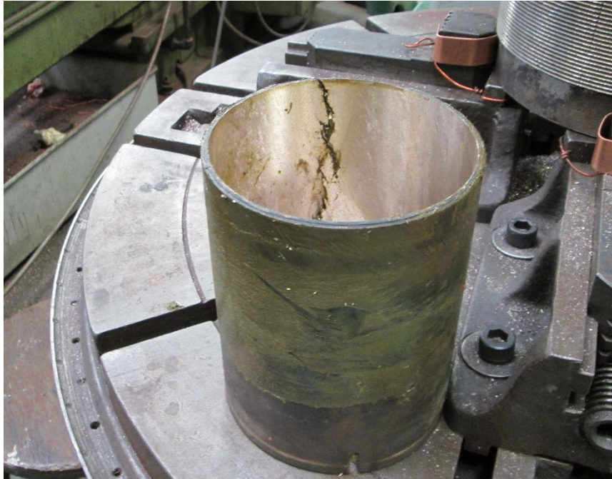
Damaged shaft bearing
