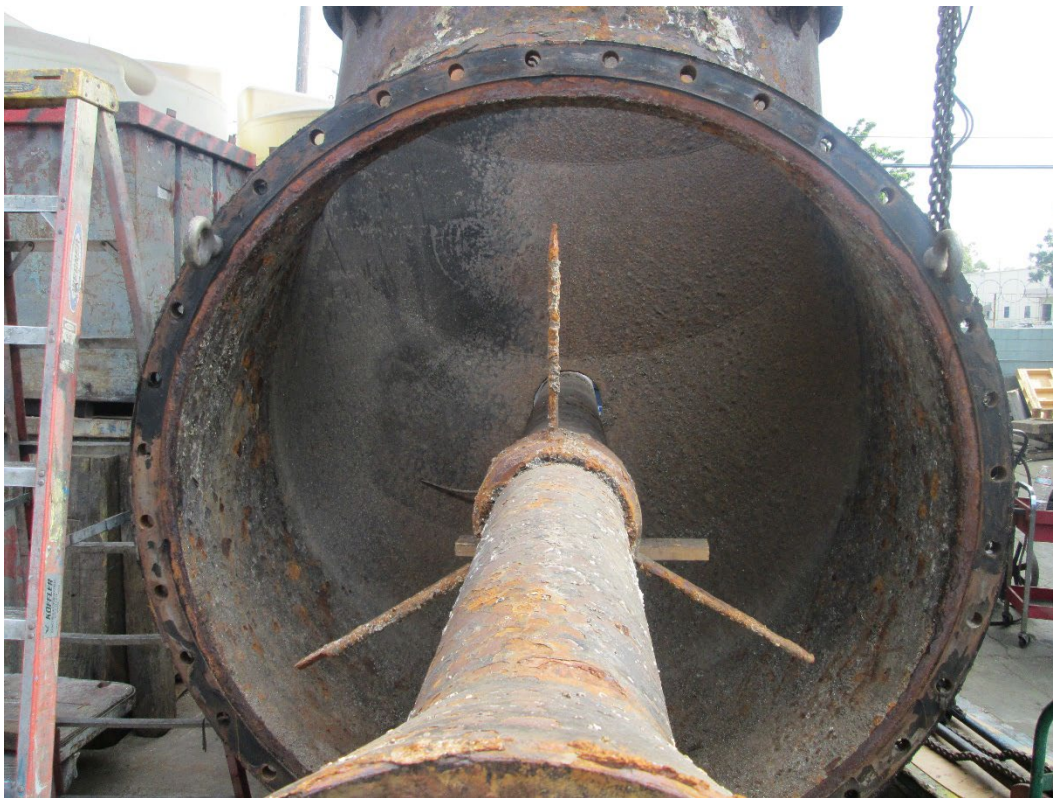
Pump discharge elbow with stabilizing spider and shaft enclosure tube
