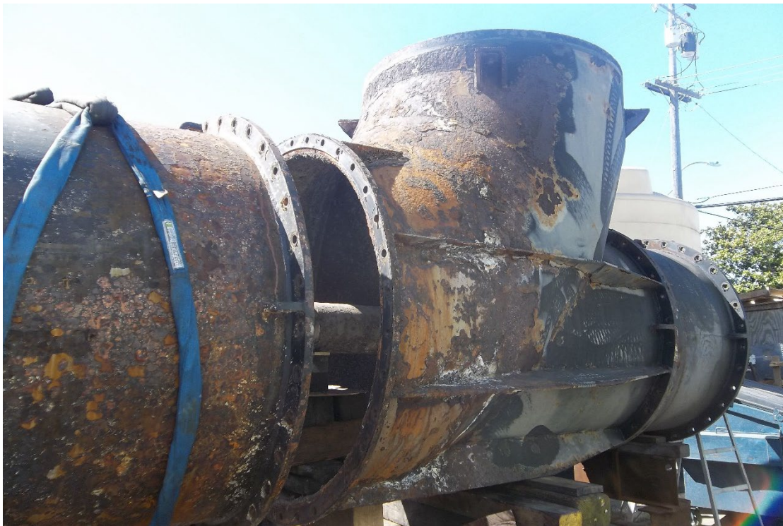
Pump discharge elbow w/ corrosion
