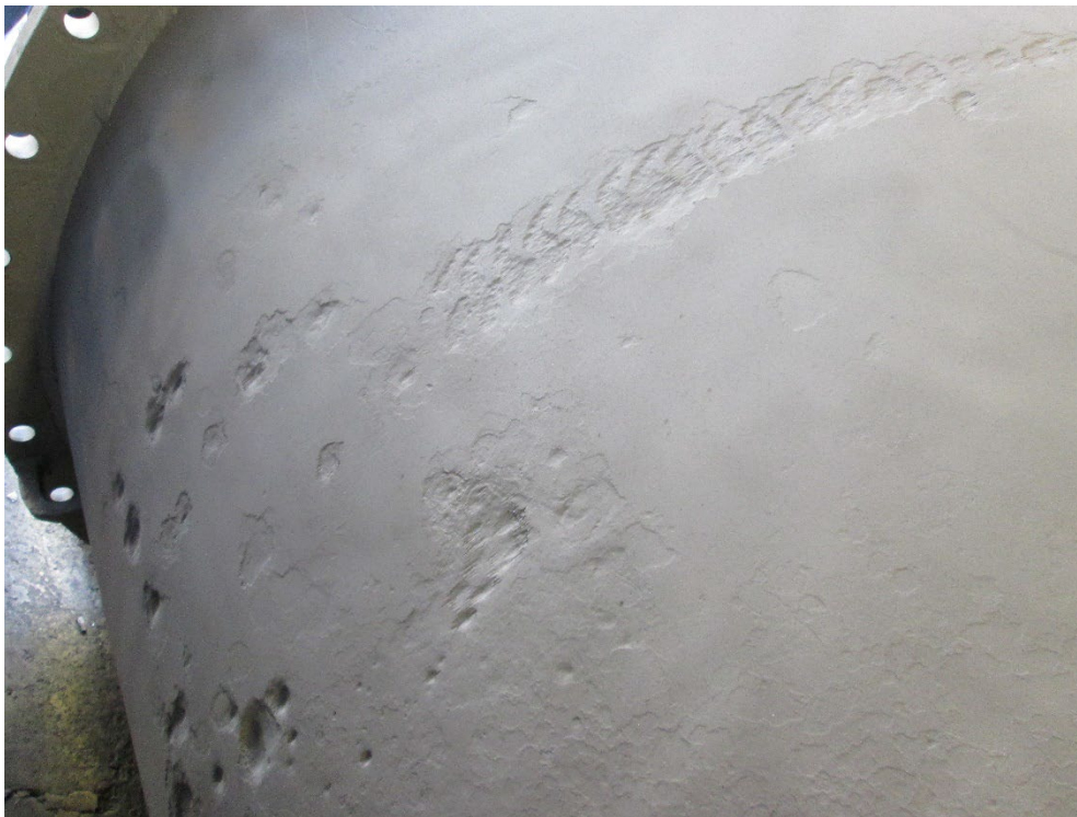
Pump column after media blasting w/ visible material loss
