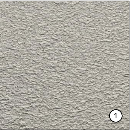
CEMENT PLASTER: SMOOTH SAND (SAMPLE FOR TEXTURE ONLY)
