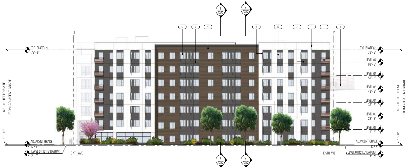
2 A302 1/16" = 1'-0" EXTERIOR ELEVATION - SOUTH - HOUSING BLOCK - STREET
