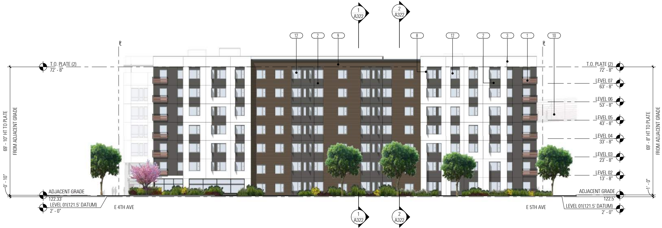
2 A302 EXTERIOR ELEVATION - SOUTH - HOUSING BLOCK - STREET 1/16" = 1'-0"
