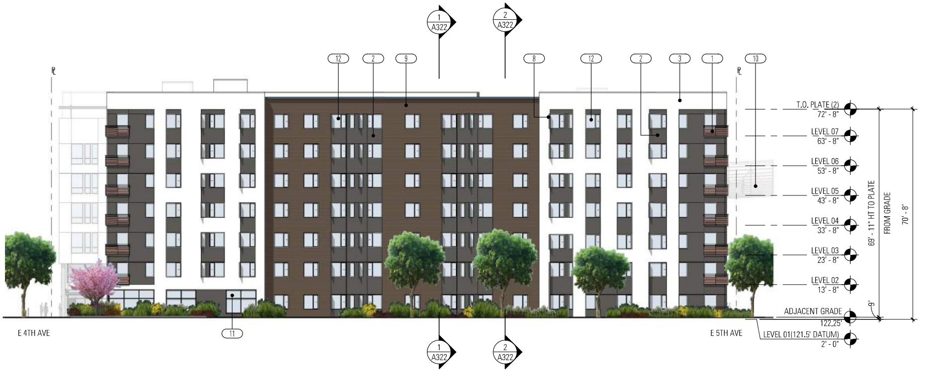
2 A302 1/16" = 1'-0" EXTERIOR ELEVATION - SOUTH - HOUSING BLOCK - STREET
