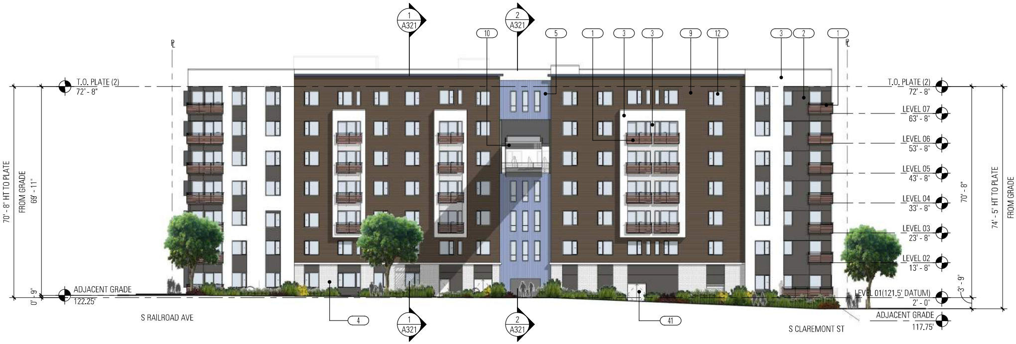
1 A302 1/16" = 1'-0" EXTERIOR ELEVATION - EAST - HOUSING BLOCK - STREET
