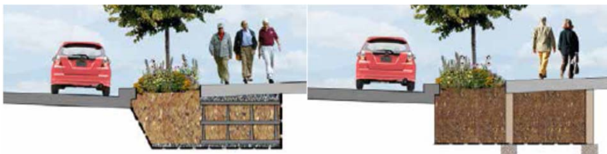
Figure 1-3. Stormwater tree well filter conceptual examples: modular suspended pavement system (left), column suspended pavement system (right). (Courtesy of Philadelphia Water Department)
