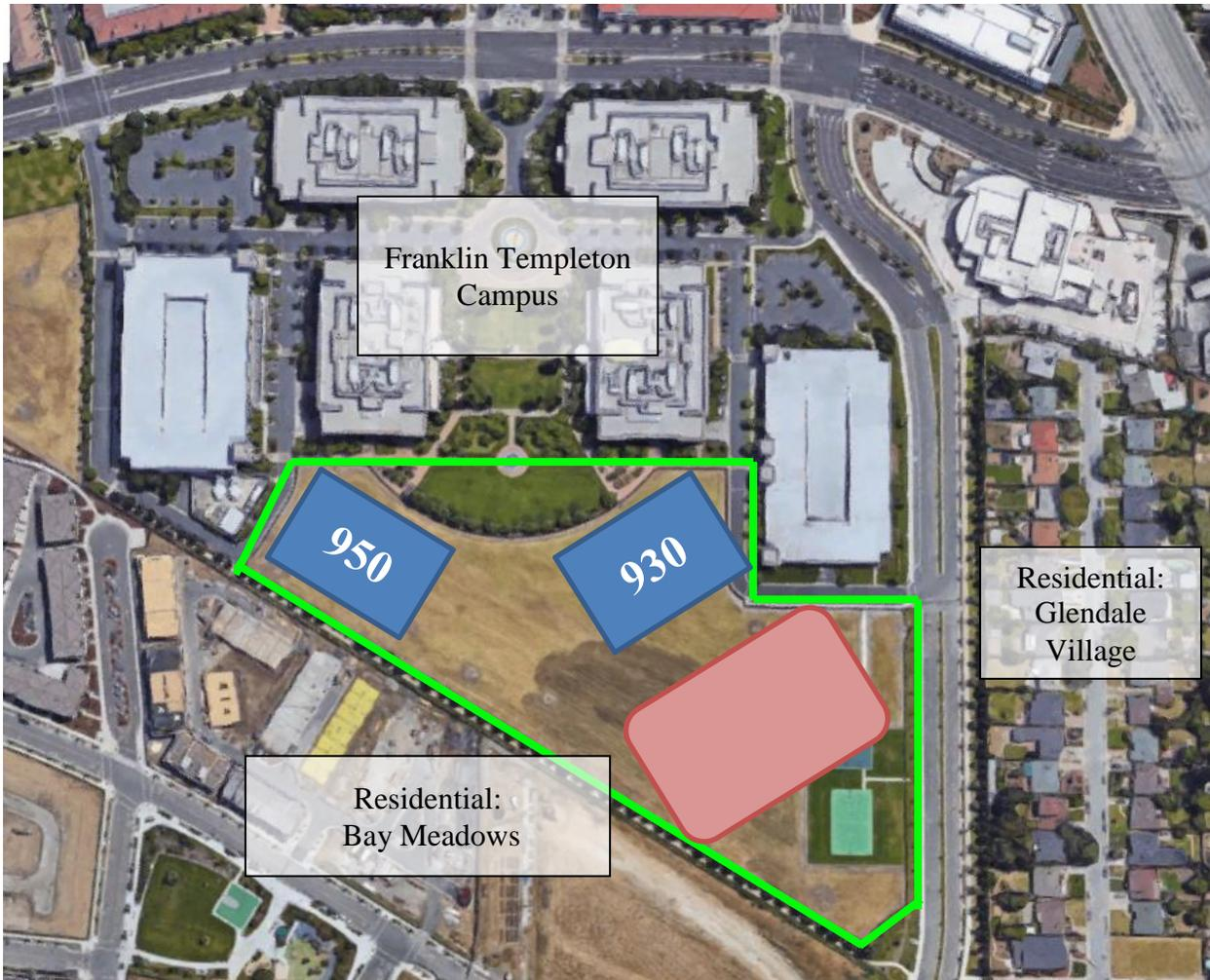
**Figure 2:** Aerial photo of project area. Construction fence outlined in green. New building locations shown in blue. New parking lot shown in red. Nearby sensitive receivers labeled on photo.
