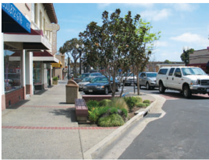
Bulbouts can extend the pedestrian realm for additional space.
