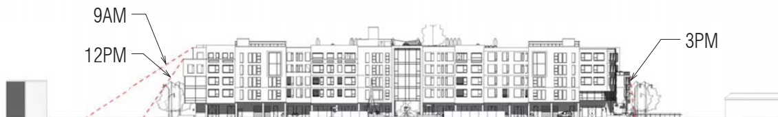
5 SOUTH ELEVATION - SPRING/FALL EQUINOX 3PM 1" = 50'-0"
