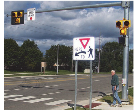
Figure 5-14: Pedestrian Hybrid Beacon (HAWK)
